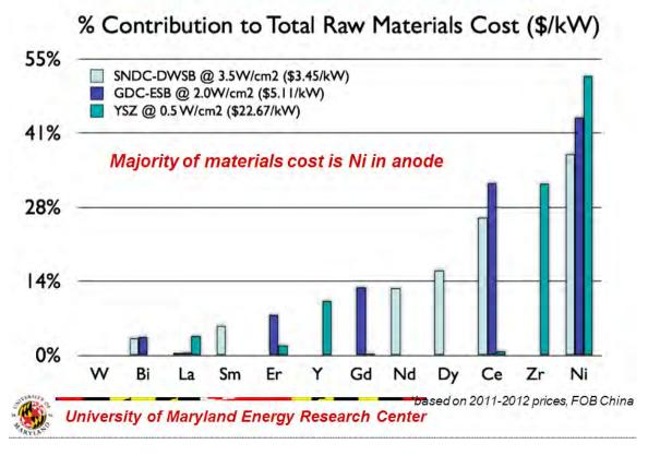
Figure 6 – SOFC relative material costs
