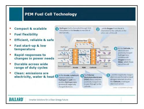
Figure 7 – proton exchange membrane (PEM) fuel cells
