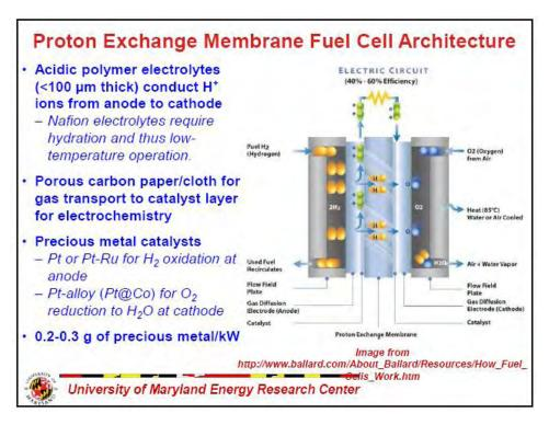
Figure 2 - Proton exchange membrane fuel cell architecture
