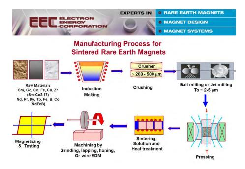
Figure 13 – Manufacturing process for sintered rare earth magnets
