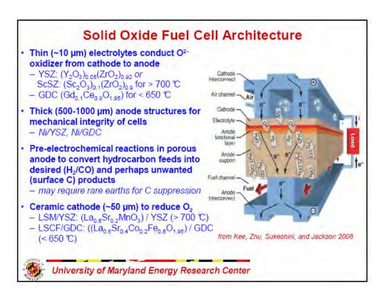
Figure 3 - solid oxide fuel cell architecture
