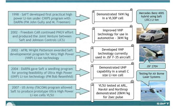
Figure 12 - Development of a practical high power Lithium Ion battery for DOD applications at SAFT
