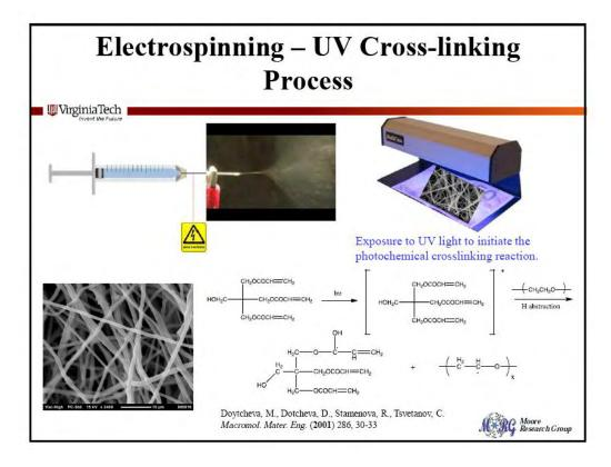
Figure 8 - Electrospinning UV light Cross-linking process
